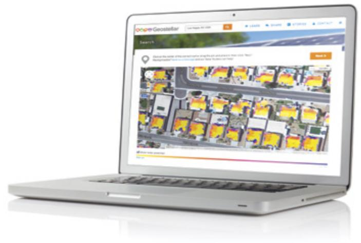
Geostellar solar potential view. Geostellar’s Search showing high-resolution solar simulations derived from LiDAR surface models and building footprints generated by eCognition.
