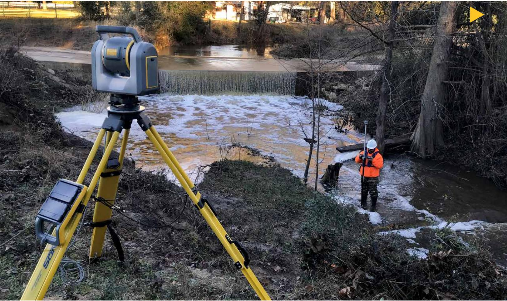
*An SOA surveyor uses the Trimble SX10 for pipeline locations.*
