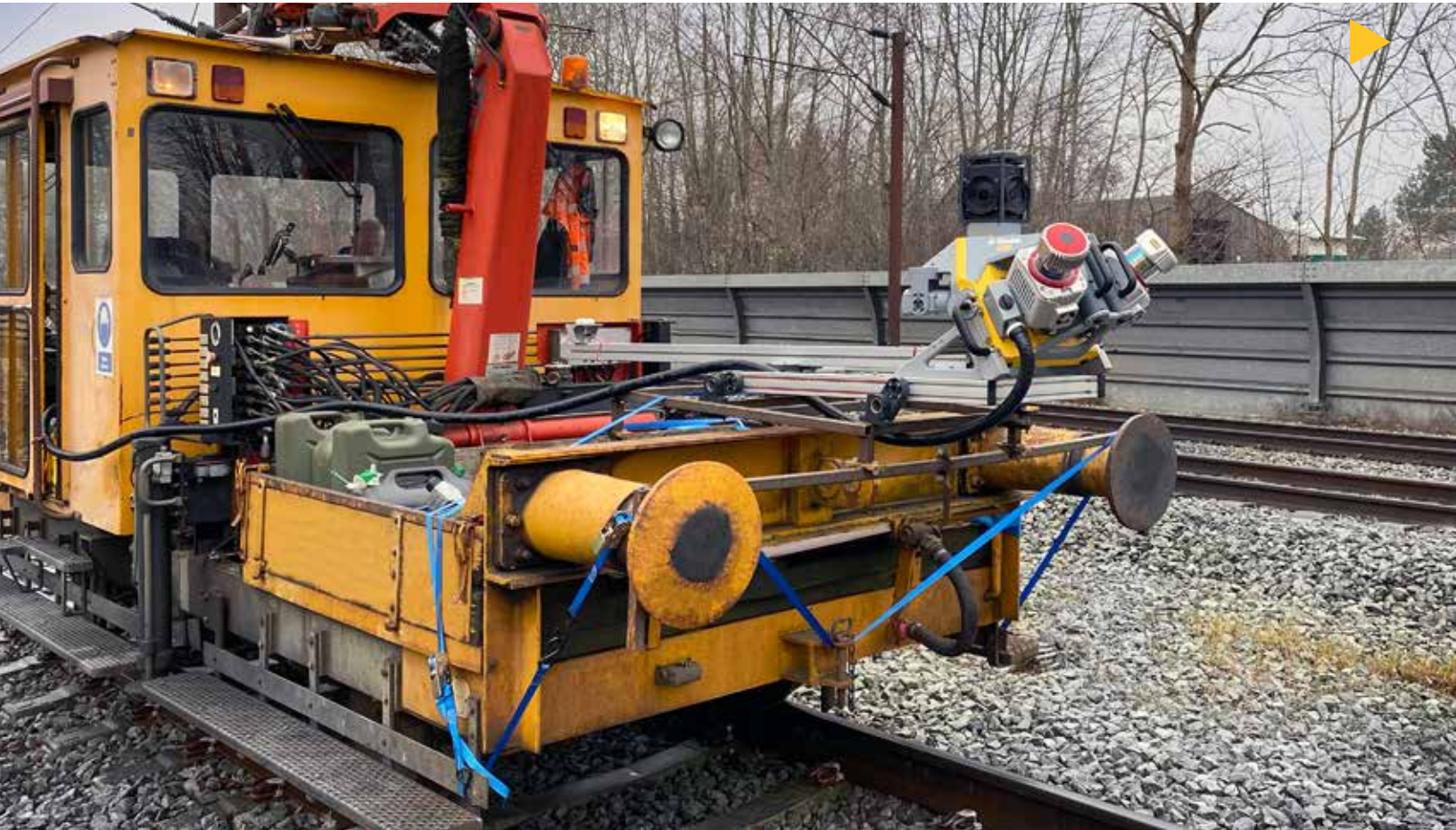
LE34 mounted the MX9 on a rail maintenance lorry for the railway mapping project. The system is controlled by a tablet computer in the lorry cabin.
