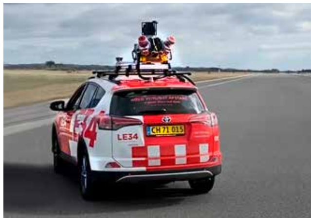
The mobile mapping system is relatively light for such instrument packages, and LE34 has adapted it for mounting on autos for roadway surveys.
